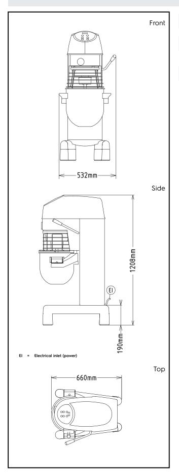
**Electric** Supply voltage: 200-240 V/1N ph/50/60 Hz Capacity: Performance (up to): 7 kg/Cycle 30 litres Capacity:
